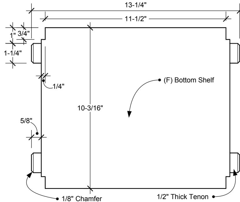
These parts are made from 3/4" thick stock.
